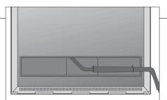
If you have a wall bracket, make sure that there is enough slack in the cables to allow the TV to turn before you fasten the cables with cable ties to make a neat bundle.
