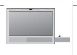
To remove the speaker cover, gently push it out using one of the four pins removed from the television. If the television is mounted on the table stand or wall bracket, you must first remove the sides on the stand or wall bracket to remove the speaker cover. See the guides enclosed with the stand or wall bracket.
